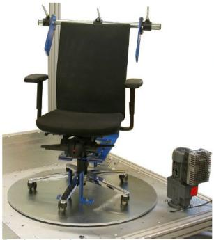
Rotation test rig for caster testing
