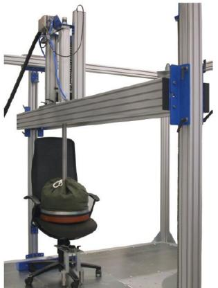
Drop tester for installation into the test field
