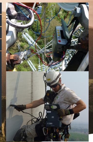
The average value is then displayed within 3 seconds, to a basic accuracy of 0.2%. DLRO 10X displays both forward and reverse measurements as well as the average of the two.
