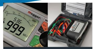
The analogue arc simulates the behaviour of a mechanical measuring needle display
