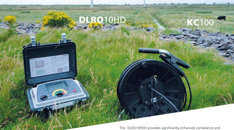
Augmenting Megger's DLRO10 and 10X range the DLRO10HDX combines ultimate simplicity of operation with a rugged IP65 case designed for stable ground and bench operation and provides memory storage.
