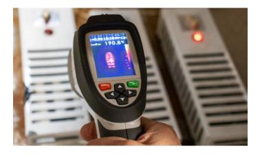
The Megger TC3231 offers a professional infrared 32 x 31 pixels image thermometer with a 2.2 inch (55.88 mm) colour TFT LCD display. Quick, accurate readings are possible; covering a wide range of surface temperature measurements.
