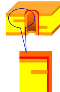
“ — ” indicates Electroless copper plating on base copper and hole wall
