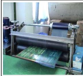
Cover entire board with semi-transparent film to mask from plating
