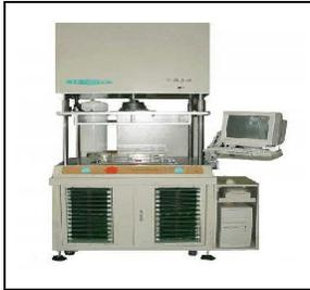
Test Fixture is developed using customer data, and will make sure finished board matches design. Test program will identify opens and shorts
