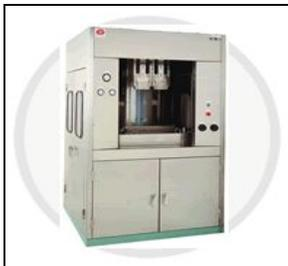
Hot Air knives blow excess solder from board surface
