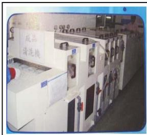
High pressure water rinse and brushes remove dust. Boards are then stacked
