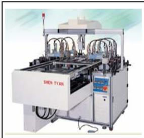
Hot copper rods melt spots to preserve layer alignment.
