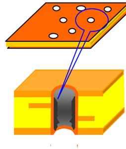
resin smear on hole wall
