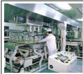
bottom copper foil placed on the press plate
