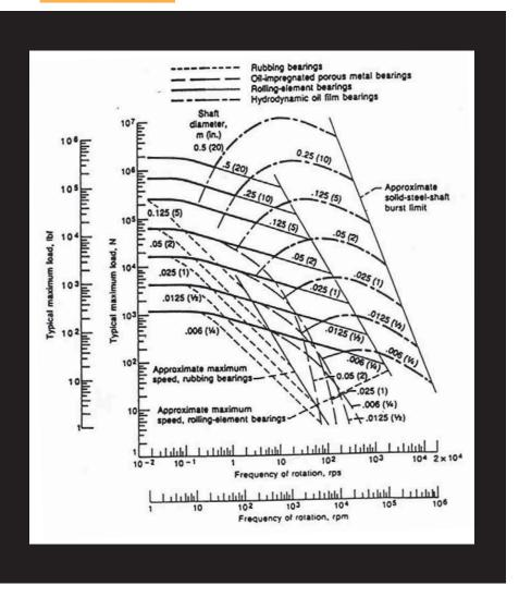
Figure 4. General guide for selecting bearings for radial loads. Bore diameters are given in inches on each curve. Except for rolling-element bearings, the length/diameter ratio = 1. Medium-viscosity mineral oil lubrication is assumed for hydrodynamic bearings. (Photo courtesy of ESDU Item 65007, Engineering Sciences Data Unit, Institution of Mechanical Engineers, London, 1965)
