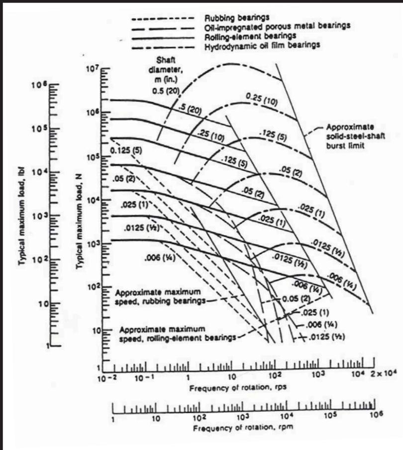
Figure 4. General guide for selecting bearings for radial loads. Bore diameters are given in inches on each curve. Except for rolling-element bearings, the length/diameter ratio = 1. Medium-viscosity mineral oil lubrication is assumed for hydrodynamic bearings. (Photo courtesy of ESDU Item 65007, Engineering Sciences Data Unit, Institution of Mechanical Engineers, London, 1965)
