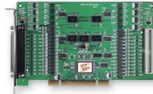
**PIO-DA16U/DA8U/DA4U****Universal PCI, 14-bit 16/8/4-ch Analog Output Board**
