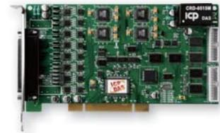
**PISO-DA16U/DA8U/DA4U****Universal PCI, 14-bit 16/8/4-ch Bus-type Isolated Analog Output Board**
