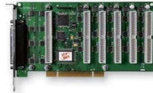
**PISO-P32C32U****Universal PCI, 32-ch Optically Isolated D/I and 32-ch Optically Isolated Open Collector output Board (Sink, NPN)**
