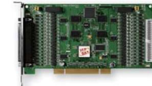
**ISO-P32S32W/PISO-P32S32WU****Universal PCI, 32-ch Optically Isolated D/I and 32-ch Optically Isolated Open Collector output Board**
