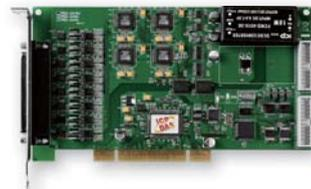
**PISO-DA2U****Universal PCI, 14-bit 2-ch Isolated Analog Output Board**
